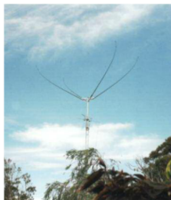
PHOTO 1: The distinctive shape of the Moxon Claw antenna explains its name.
